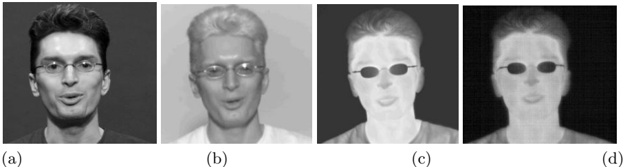
Figure 6.2. A face simultaneously imaged in the (a) visible spectrum, 0.4\text{--}0.7\ \mu\text{m} , (b) shortwave infrared, 0.9\text{--}1.7\ \mu\text{m} , (c) midwave infrared, 3.0\text{--}5.0\ \mu\text{m} , and (d) longwave infrared, 8.0\text{--}14.0\ \mu\text{m} .
