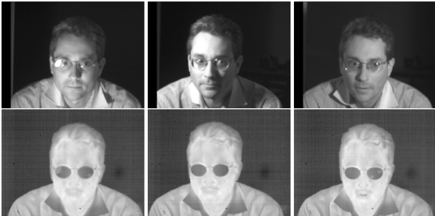
Figure 6.5. A qualitative demonstration of the illumination invariance for LWIR imagery of a face under different illuminations. Top row: Visible imagery of a face under three illumination conditions respectively front, left, and right. Bottom row: Co-registered thermal IR imagery simultaneously acquired for each of the three images in top row respectively.
